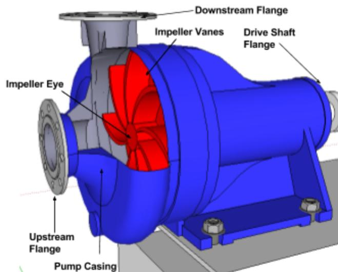
2. According to the above diagram, which part of the centrifugal pump does the motor connect to?
